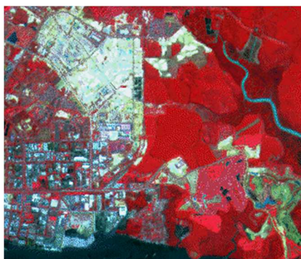
False colour composite multispectral SPOT image: Red: XS3; Green: XS2; Blue: XS1
